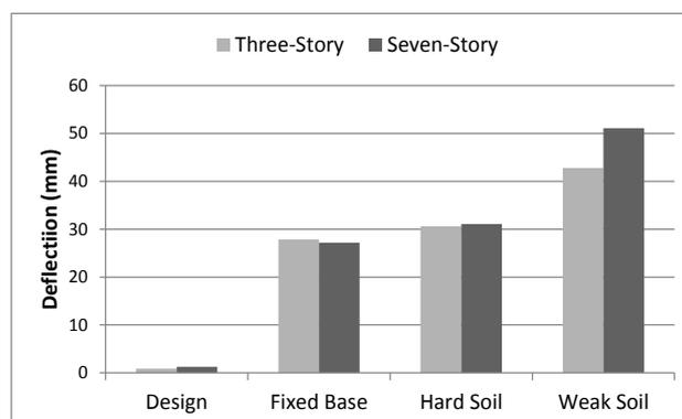
**Fig.5. Deflection at point of column removal – Linear Static Analysis**
