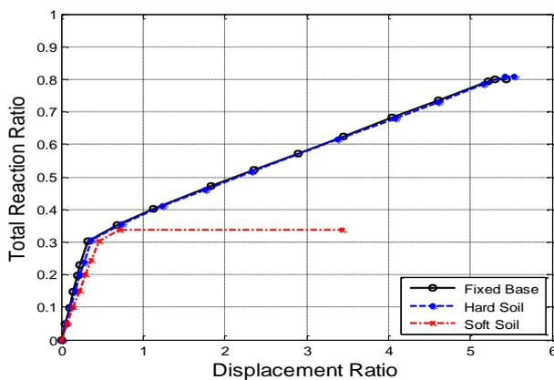
Fig.23 Total Load – Deflection relation for Edge Roof-Floor Column Removal of the Seven-Story Building
