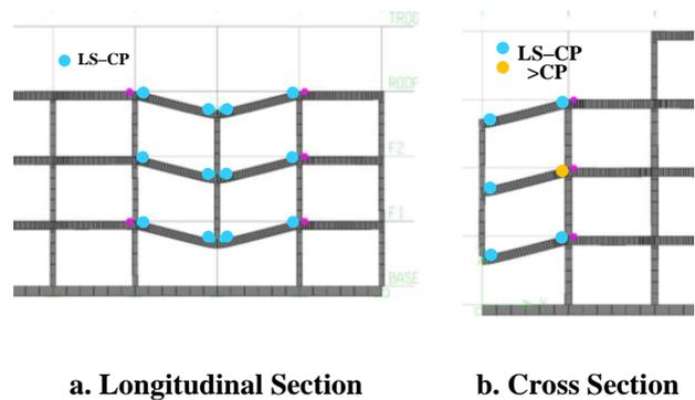
Fig.7. Plastic Hinge Formation in the Three-Story Building for Edge Ground-Floor Column Removal, Fixed Base
