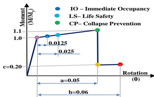
Fig.1. Moment curvature properties of plastic hinge
