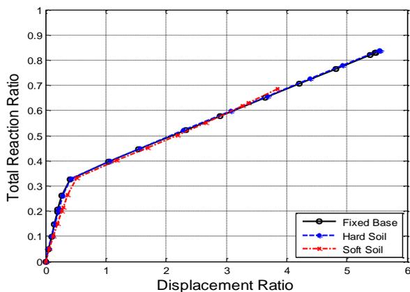
Fig.8 Total Load-Deflection relation for Edge Ground-Floor Column Removal of the Three-Story Building
