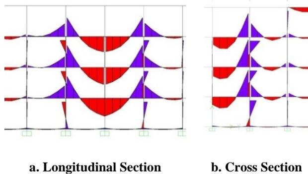
Fig.6. Three-Story Building Moment for Ground-Floor Column Removal, Fixed Base
