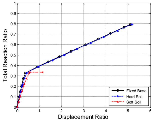
Fig.20 Total Load – Deflection relation for Edge Mid-Floor Column Removal of the Seven-Story Building
