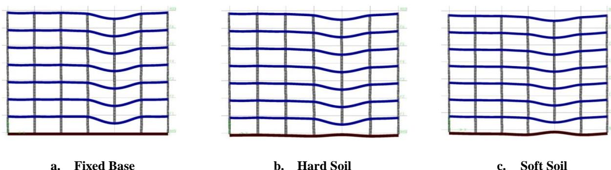
**Fig.4 Deformed Shape of The Seven Story Building**
