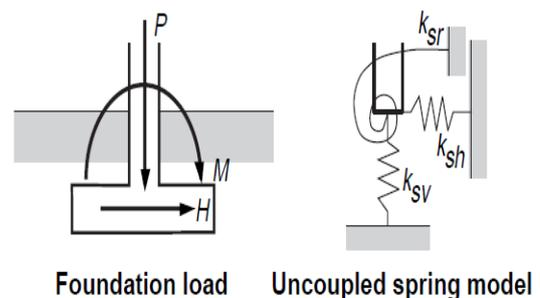
Fig.2. Uncoupled Spring Model [21]
