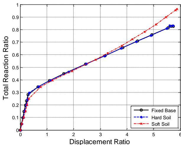
**Fig.14 Total Load – Deflection relation for Edge Roof-Floor Column Removal of the Three-Story Building**
