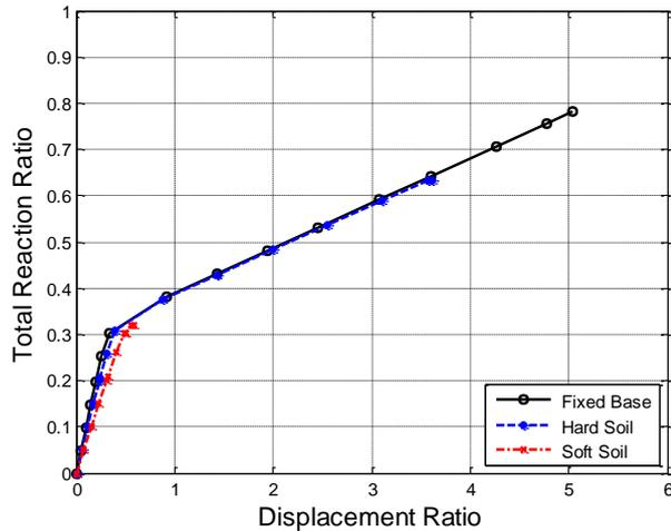
**Fig.17 Total Load – Deflection relation for Edge Ground-Floor Column Removal of the Seven-Story Building**
