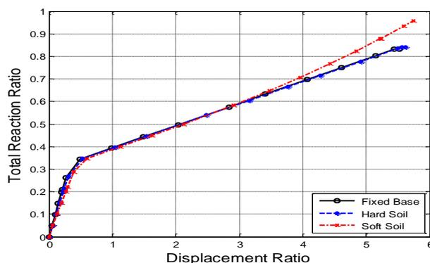
**Fig.11 Total Load – Deflection relation for Edge Mid-Floor Column Removal of the Three-Story Building**
